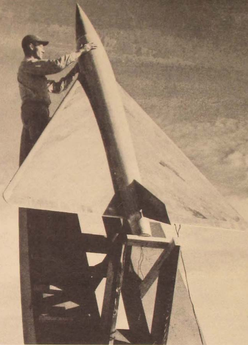
A delta-wing research model is prepared for firing at NACA's pilotless-aircraft test station on Wallops Island, Virginia. This large wooden model, designed to measure drag on a delta wing, is powered through transonic speeds by an internal rocket.
